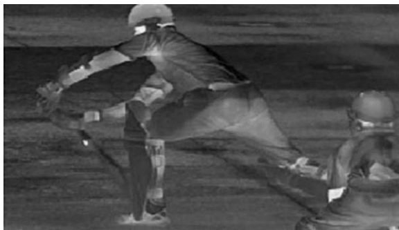
Fig. 1. Hotspot in Cricket. A spot is detected on the bat because of the temperature change detected by thermal imaging.
